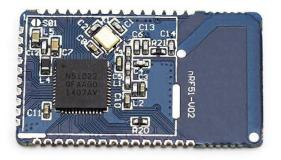
nRF51822 series 2.4 GHz transceiver, a 32 bit ARM® Cortex<sup>™</sup>-M0 CPU, flash memory, and analog and digital peripherals. nRF51822 can support Bluetooth® low energy and a range of proprietary 2.4 GHz protocols, such as Gazell from Nordic Semiconductor.
